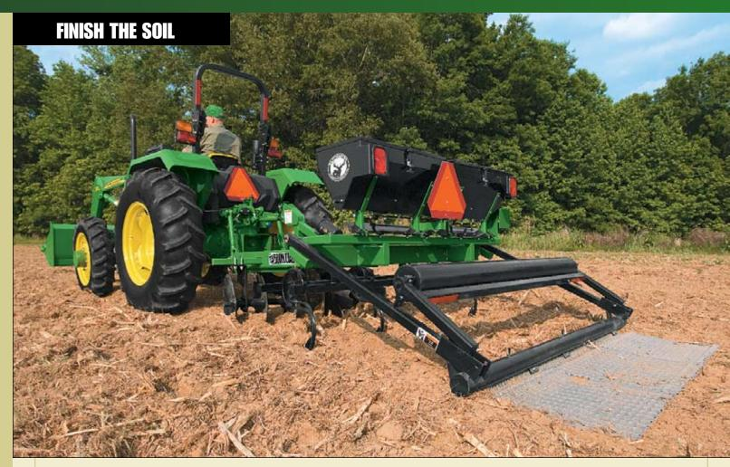
Once the seed hits the ground, the flexible metal grating drag levels the soil and covers the seed for uniform soil contact. You can choose between three covering options. Drag only, drag with roller on top and roller only. The FP1206 and FP1208 feature a handle to easily flip the roller over.
